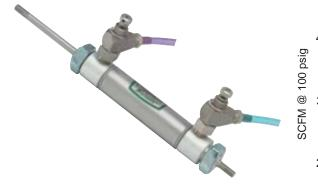
Clippard offers five models of adjustable flow controls with #10-32 through 3/8" NPT ports. They feature a combination needle and check valve that controls flow in one direction and allows free flow in the opposite direction.
